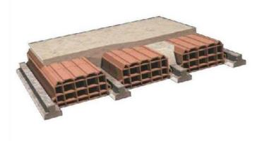
2. Slab with brick blocks and joists: the thickness considered for this layer is equal to 30 centimeters while as regards the conductivity coefficient this has been taken equal to 0,7  $W/m*^{\circ}C$
